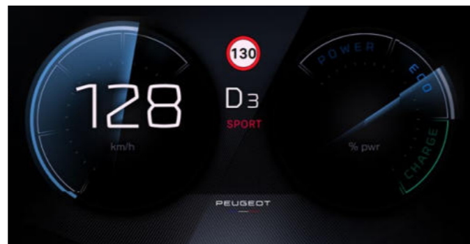
The digital speedometer (image shown is for 208 ELECTRIC variants, displaying numbers in metric system.)
